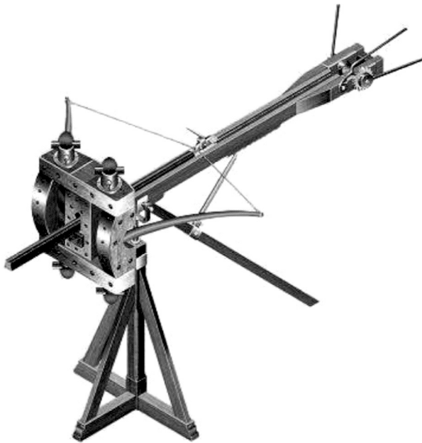
Fig. 3. Pictorial reconstruction of the ballista of Vitruvius. Adapted from [2]
