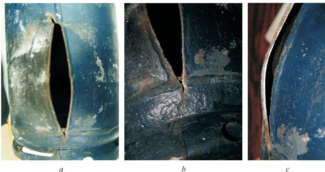
Figure 3. The LPG cylinder after the BLEVE explosion, the 170 mm fractured cylinder lateral weld, the lower dome peripheral weld (a), corrosion defects and corrosion pits at the lower dome (b) and lateral cylinder weld penetration 1.10–1.50 mm out of the 2.80 mm shell thickness at a length of 40 mm (c)
