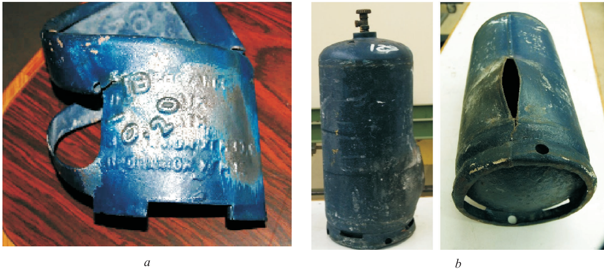
Figure 2. The LPG cylinder after the BLEVE explosion, the upper protection, year of construction 1965, pressure test 2 MPa (a), cylinder length 400 mm, diameter 250 mm, spherical bottoms height 60 mm, radius of curvature R = 280 mm, and the weld failure (b)
